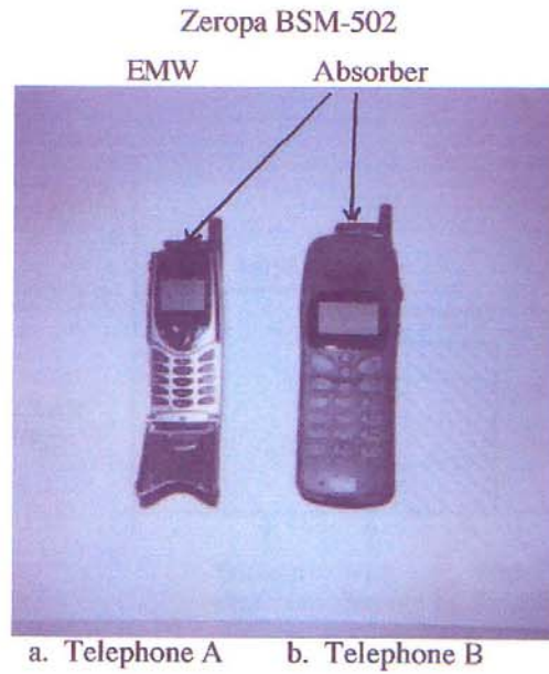
Fig. 1. Photograph of the two cellular telephones A and B with Zeropa BSM-502 EMW absorber samples mounted on top at base of the antenna.
